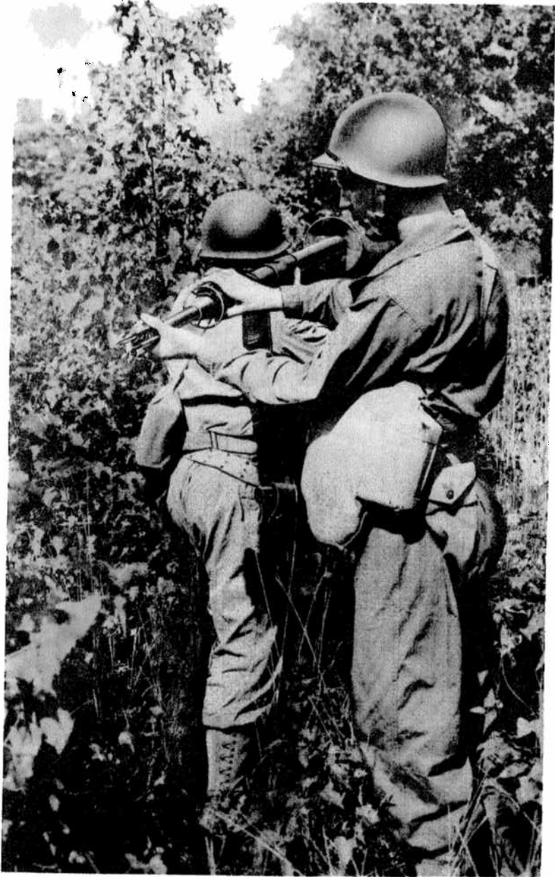
Figure 3 — Loading Rocket Into Launcher
